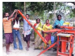
Compressed brick making
